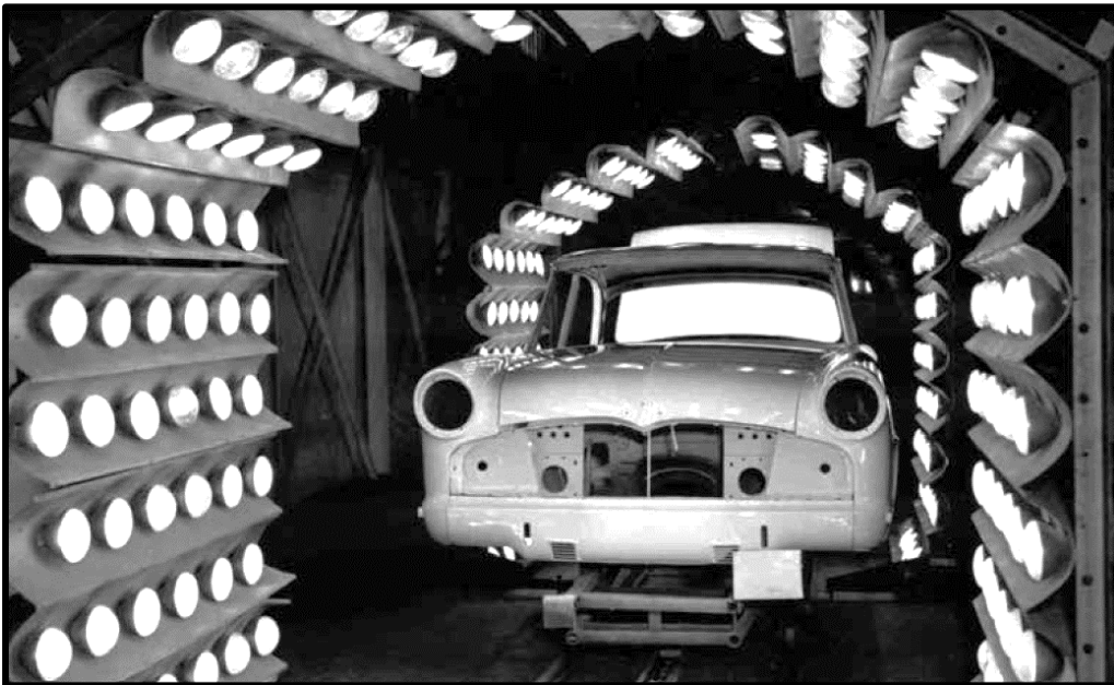
A Simca Vedette going through a drying booth at the paint shop back in the day.
